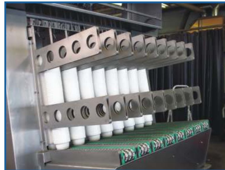
Becherpuffermagazin Cup buffer magazine
