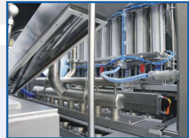
Bechersterilisation (UVC-Strahler) Cup sterilisation (by uvc-high power heater)
